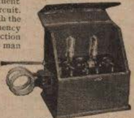
Illustration of S.T.100 in fine double-drop front oak cabinet with valves enclosed and batteries at rear.
